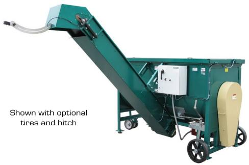
The Twister II Pro Batch Mixer can mix a wide variety of materials such as sand, peat, bark and soil, as well as chemicals and fertilizers.
