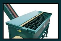
Incline conveyor for loading into various machines
