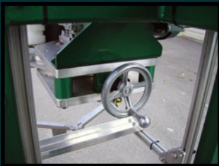
One adjustment for different pot sizes
