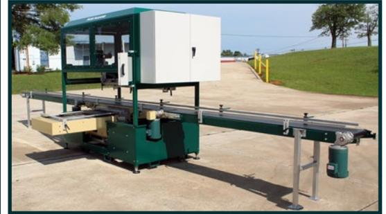
The B&L PlugPlanter M or S model offers fast accurate planting, quick change-over and CNC operating system for one of the easiest, quickest setups available. Quick-change grippers for easily switching plug size and push-up pins to ensure soft or young plugs are extracted and planted without damage. The PlugPlanter gives you flexibility to use your plug tray widthwise or lengthwise on the same machine to match container and plug tray count in the most efficient way.
