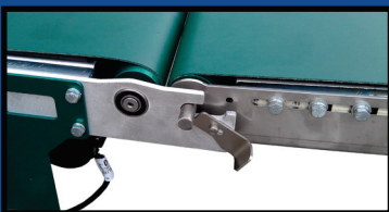
Conveyor to conveyor interlocking system
