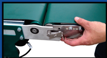
Conveyor to conveyor interlocking system
