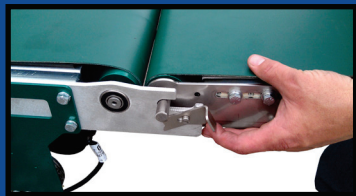
Conveyor to conveyor interlocking system
